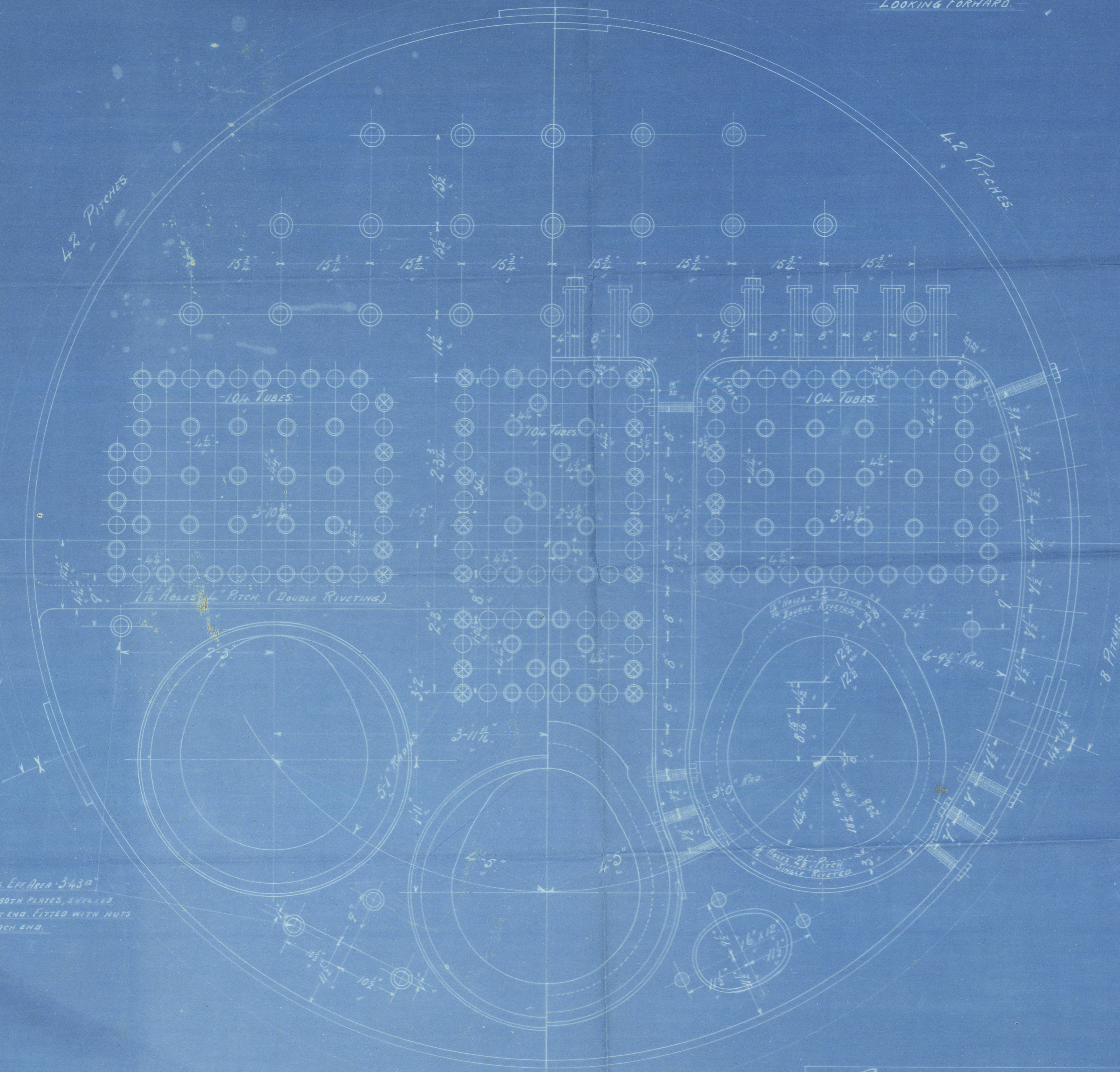
POSITION OF MANHOLES ON BACK OF BOILERS LOOKING FORWARD
