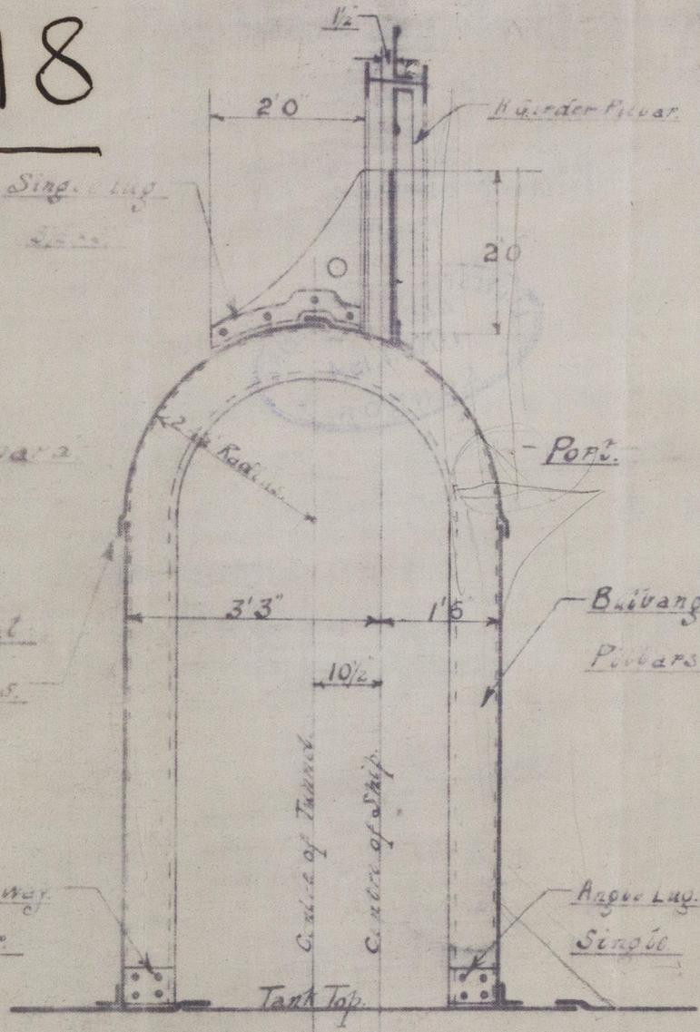
Fig A. Knice lapped on Bulb
