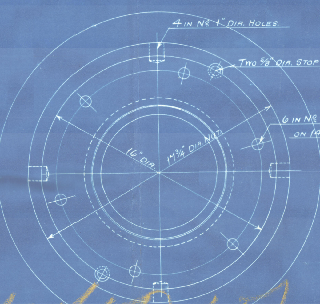
END VIEW OF STERN TUBE & NUT.
