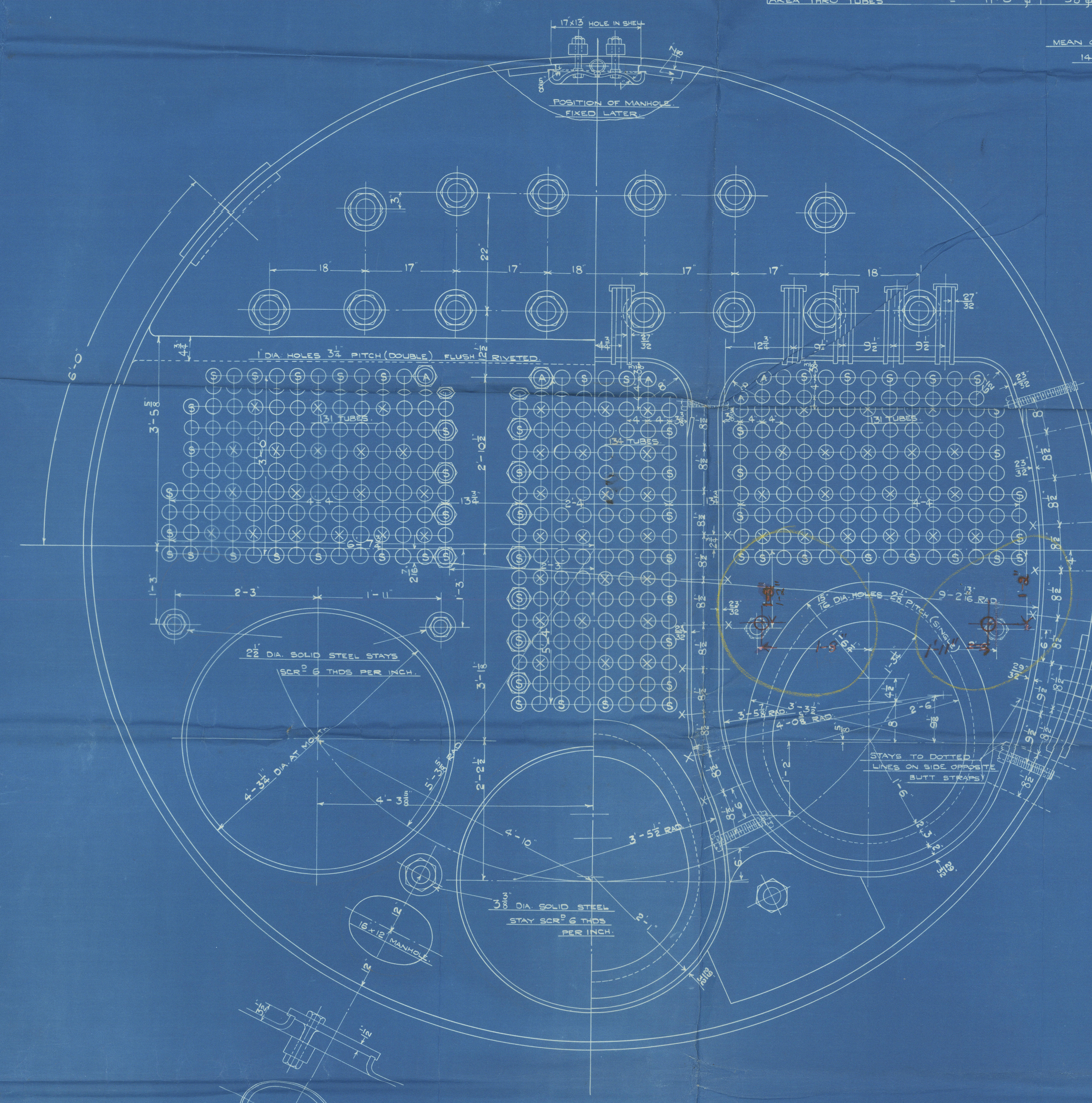
HAWTHORN-GRAY PATENT COMPENSATING PLATE 8 DOOR SEE STD. DRS. NO. 1495.
