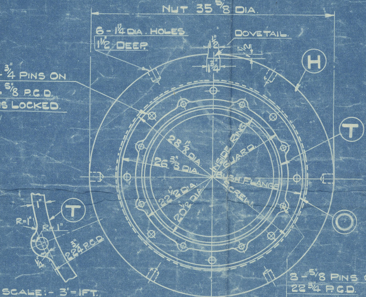
STERN TUBE NUT BUSH FLANGE AND GUARD RING. LOOKING FORWARDS. SCALE: 3" = 1 FT.
