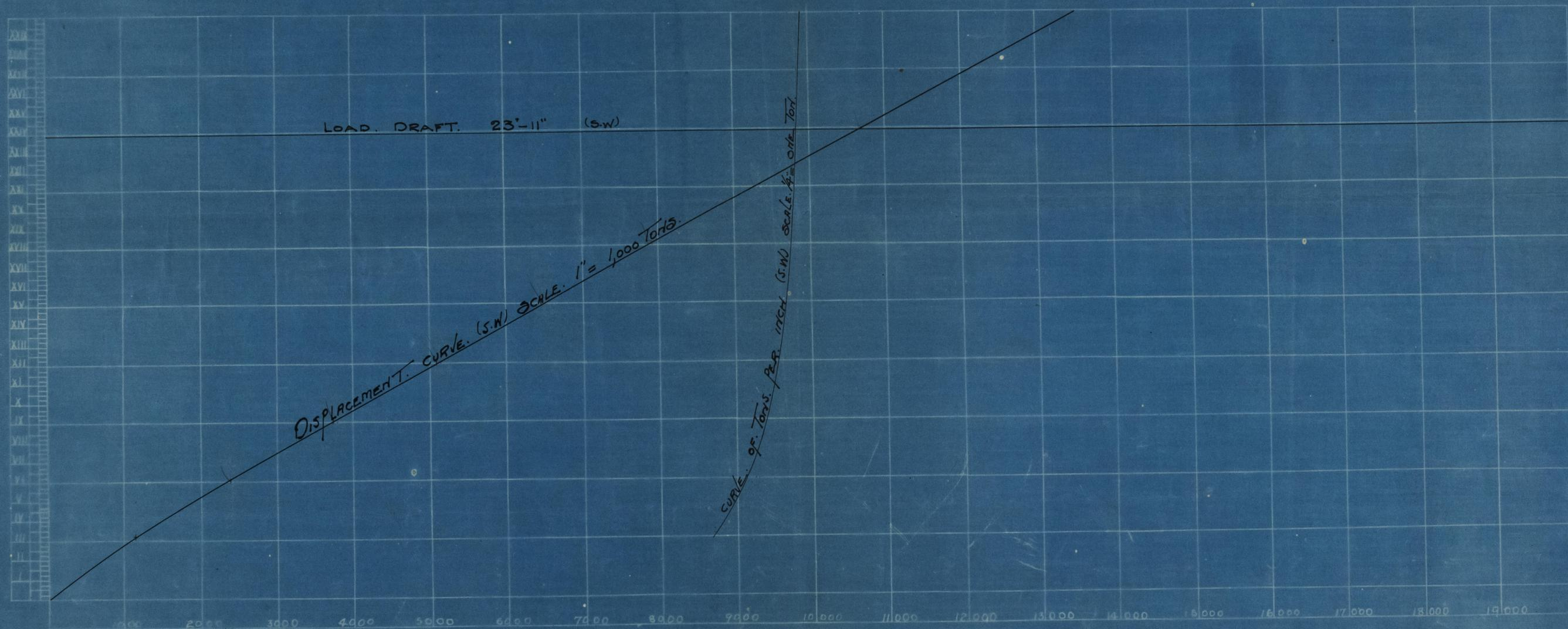
DISPLACEMENT AT L<sup>y</sup>. W.L (23'-11" S.W.) = 10680 TONS
