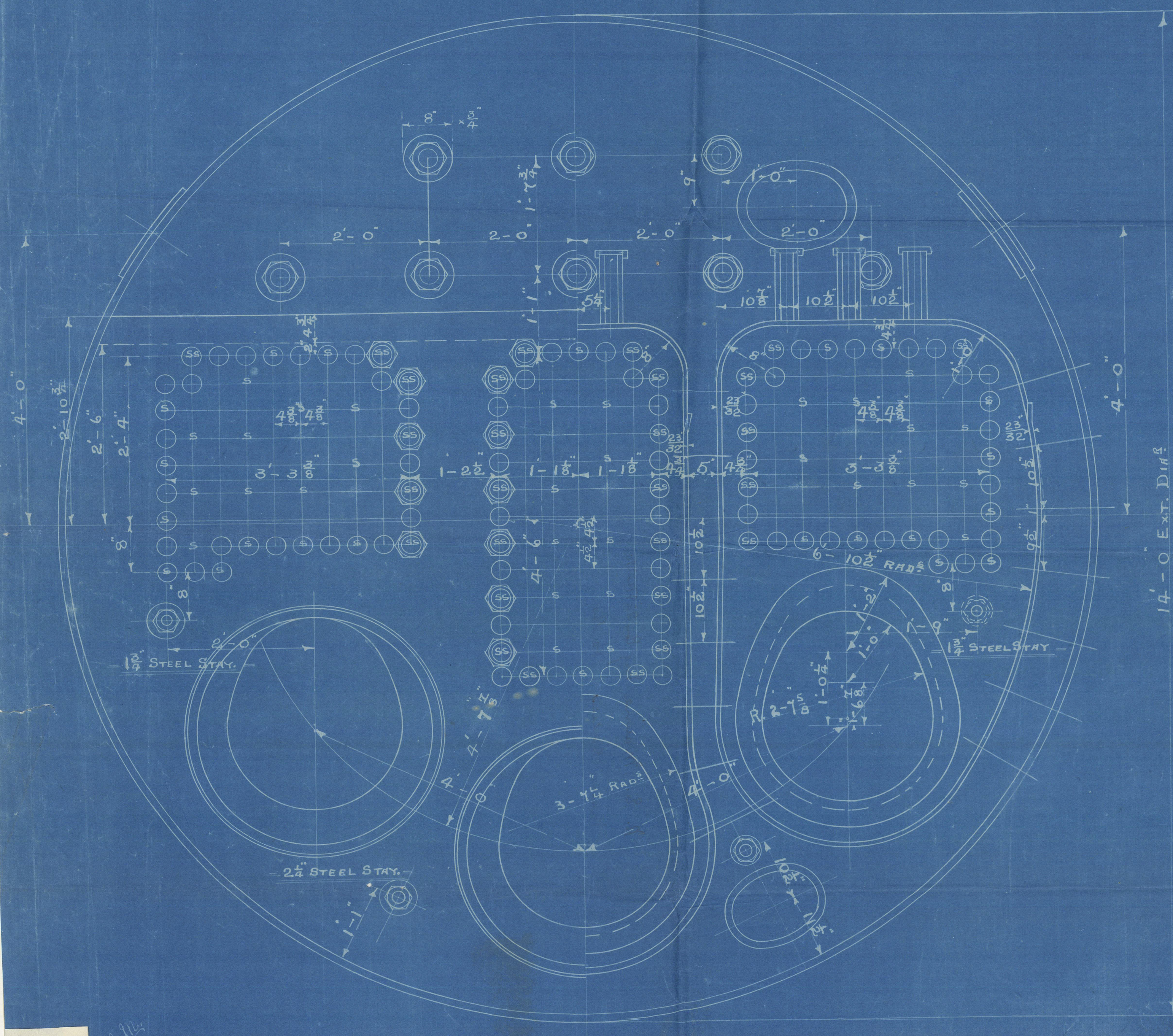
VIEW LOOKING ON BACK OF BOILERS SHOWING POSITION OF MANHOLES AND BUTT JOINTS.
