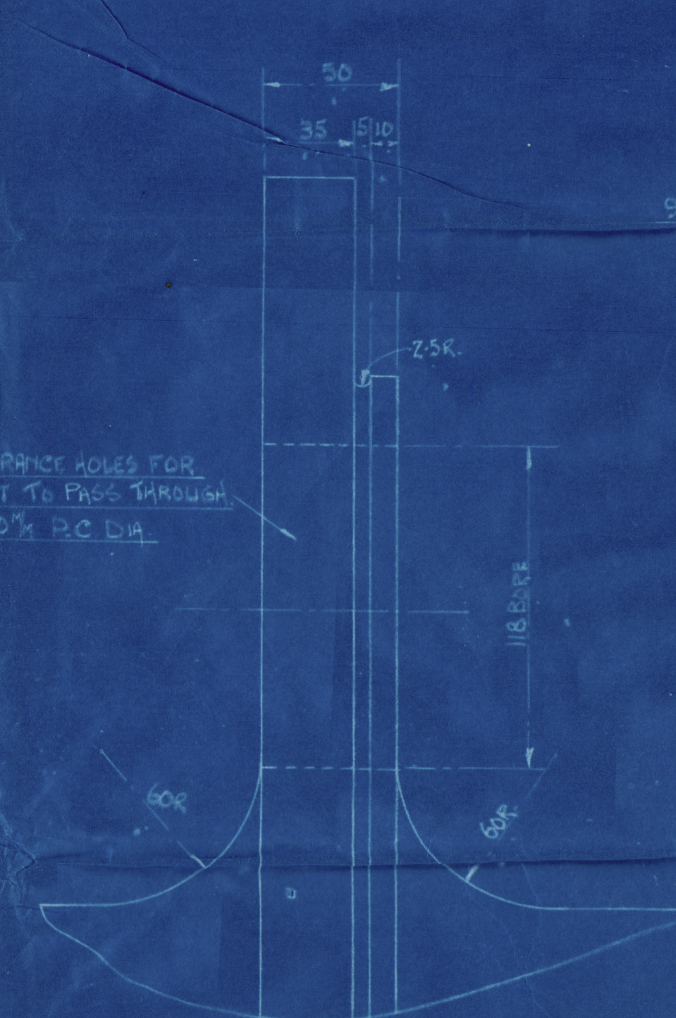
SPIGOT FOR GEARWHEEL
