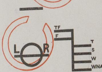
THIS IS TO CERTIFY that this ship has been surveyed and the freeboards and load lines shown above have been assigned in accordance with the Convention.
