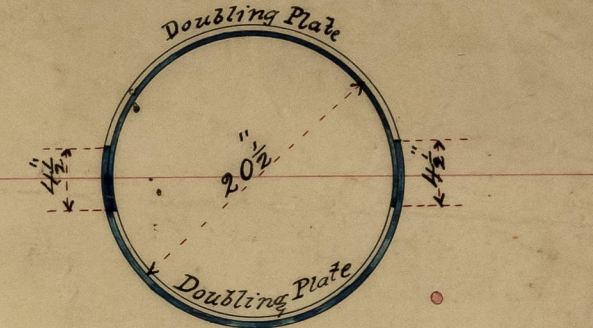
Section thro Main Mast at Height of Quarter Dk.
