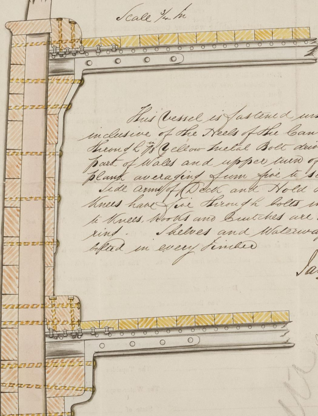
This vessel is fastened with Yellow Metal inclusive of the Heels of the Cant Timbers, also a Row of Yellow Metal Bolt driven between upper part of Wale and upper turn of Bilges in each plank averaging from six to seven feet apart. Side arms of Deck and Hold Beam hanging knees have six through bolts in each, all bolts to knees. Woods and Butches are driven on a Copper ring. Shelves and Waterways are through fitted in every timber.
