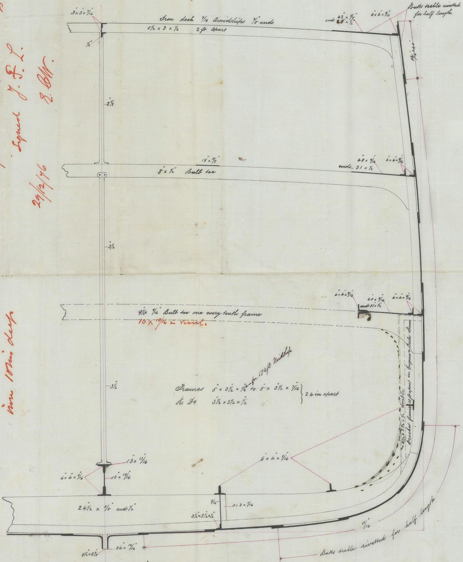
Note: This is exact copy of Scantlings submitted Dec 19<sup>th</sup> 76, with modifications in Scantlings as required per letter and App. and now being worked to as modified. L. Laidson
