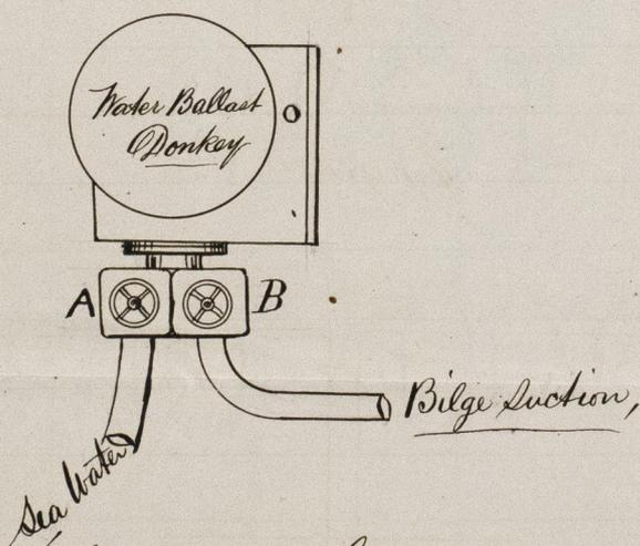
Water could be run into ship by opening the Valve B. whilst the Valve A and its sea Connections are open,
