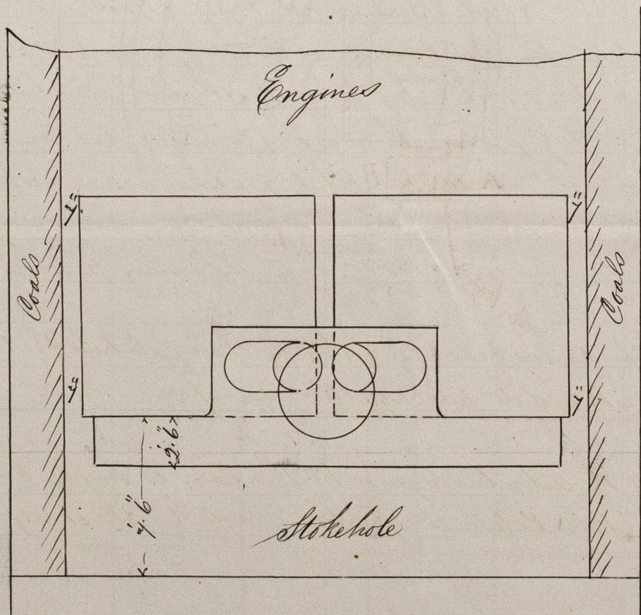
Boilers Covered with Composition & lead on top of it
