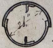
plates 11.10 long and 1/8 thick Foremast 25 feet long
