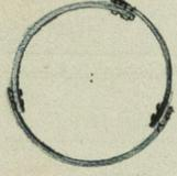
Fore & main masts of 8/16 plate at wedging tapered to 7/16 at head & hubs made with three plates, double rivetted at edges & butts with 3/4 rivets spaced 2 3/4 in, laps of edges 4 in. length 80 & 90 ft. respectively, length of plates 9 ft. Diameter at wedging 32 head 22 & head 26 in. Main mast of 7/16 plate at wedging tapered to head & hubs. ANCHORS, and their weights.
