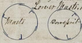
Lower Mast, Bowsprit, Lower Yard, & Lower topsail Yards of Iron, best boiler plate, Fore & Main Mast 3 1/2 inch thick, three angle irons 3 1/2 x 3 1/2 x 1/4 in each about 40 feet long, Mizzen Mast plate 5/8 inch thick, three angle irons 3 1/2 x 3 1/2 x 1/4 in, about 35 feet long, Bowsprit plates 3/8 inch thick, two angle irons 3 1/2 x 3 1/2 x 1/4 in for entire length. Butts double, treble & quadruple rivetted where strength is most required, 3/4 inch
