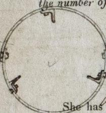
Fore main & Mizzen Masts of 7/16 plate at wedging tapered single rivetted at edges double do. at butts with 3/4" plates inside 3 1/2 x 3 x 1/16. Bowsprit 7/16 plate single rivetted four angle Irons inside 4 x 3 x 7/16. Fore & main Yards 6/16 plate at center
