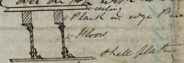
In what manner are the surfaces preserved from oxidation? Inside Plat cemented with Portland cement other parts with Ditto ditto Outside With three coats of paint
