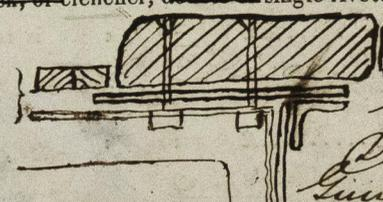
Waterway " " planksheer and to the Beams (if necessary). bolted down to Deck Beams & Gunwale Stringer Plate
