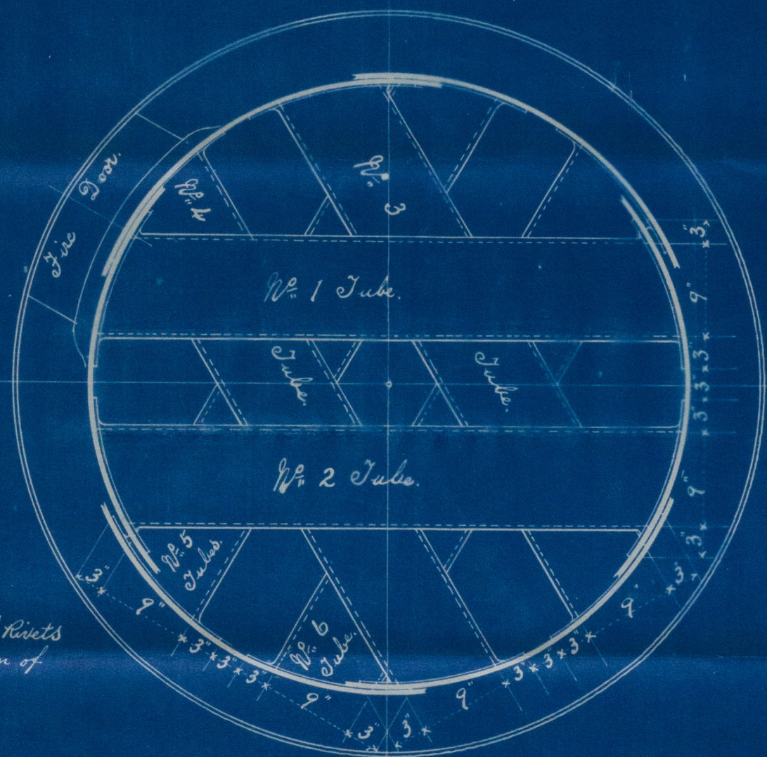
Section showing Tubes
