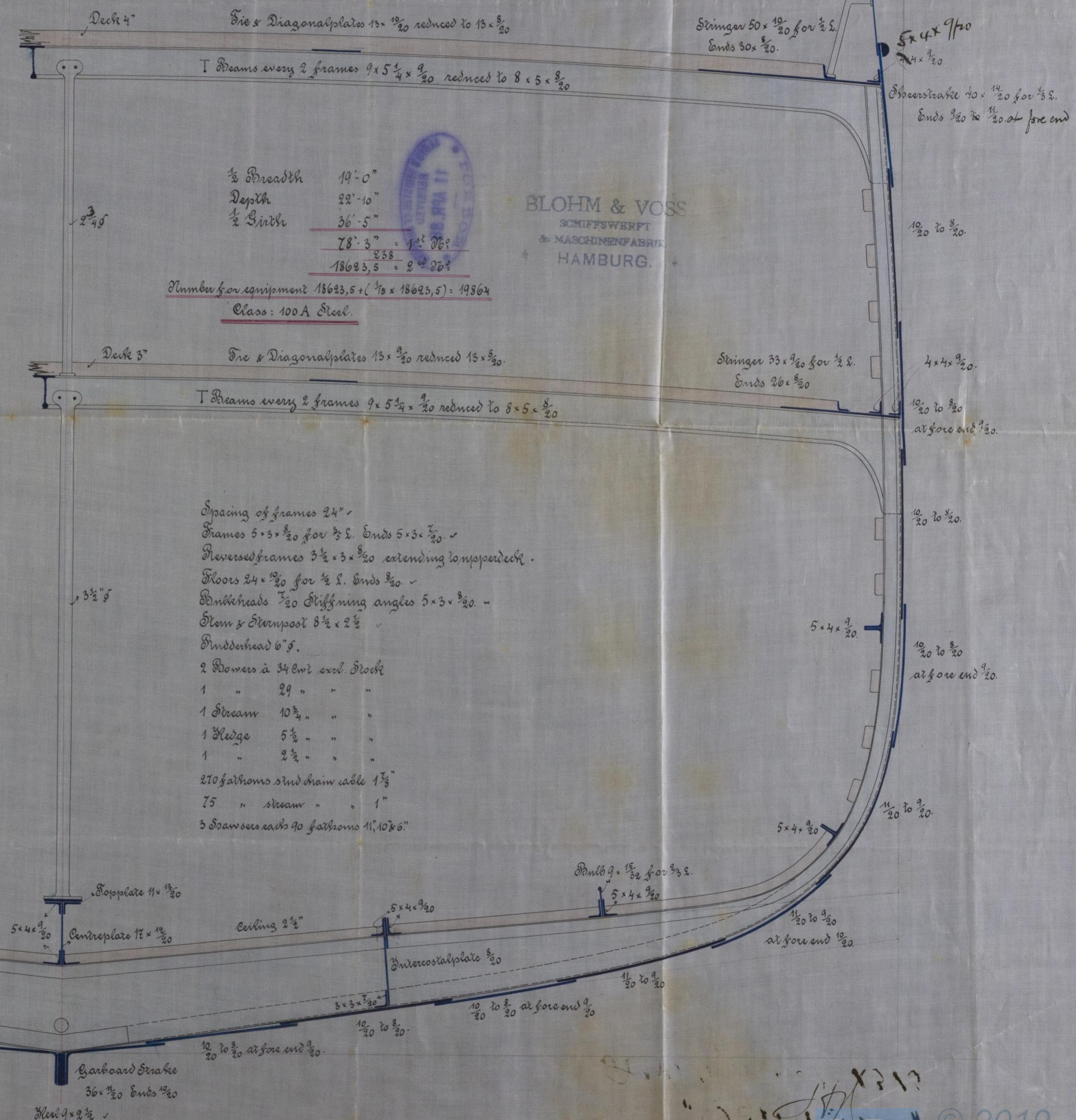
All landings of outside plating to double riveted.
