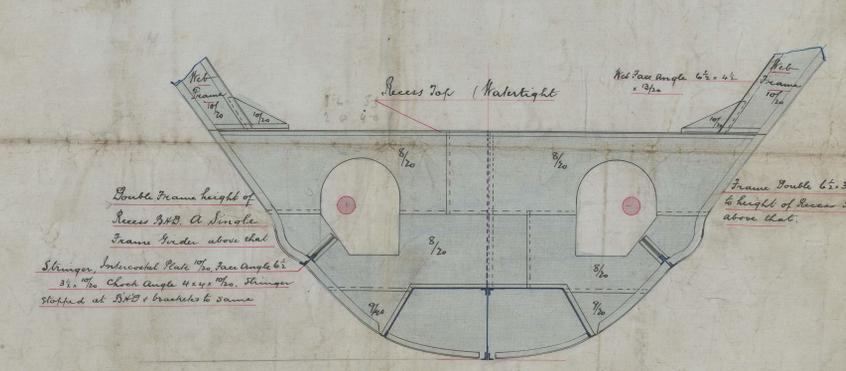
Frames all of 81 to be built to Main 88. 5 1/2 x 3 1/2 x 7/16 Bosses Part built as shown in sectional elevations Bosses Frame 6 1/2 x 3 1/2 x 7/16
