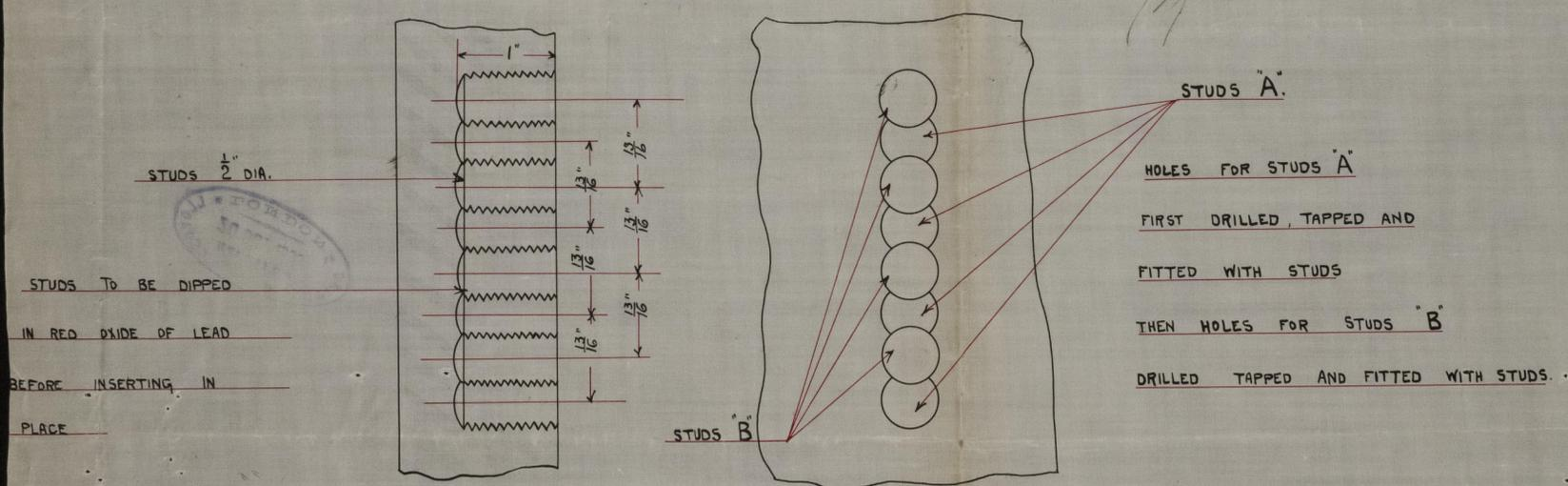
SKETCH SHEWING METHOD OF FILLING CRACKS
