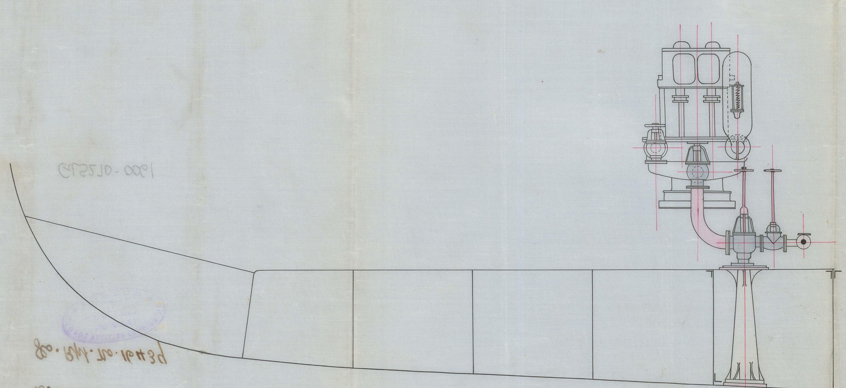
SECTION AT 91 LOOKING FORWARD ASH-EJECTOR SEA SUCTION.
