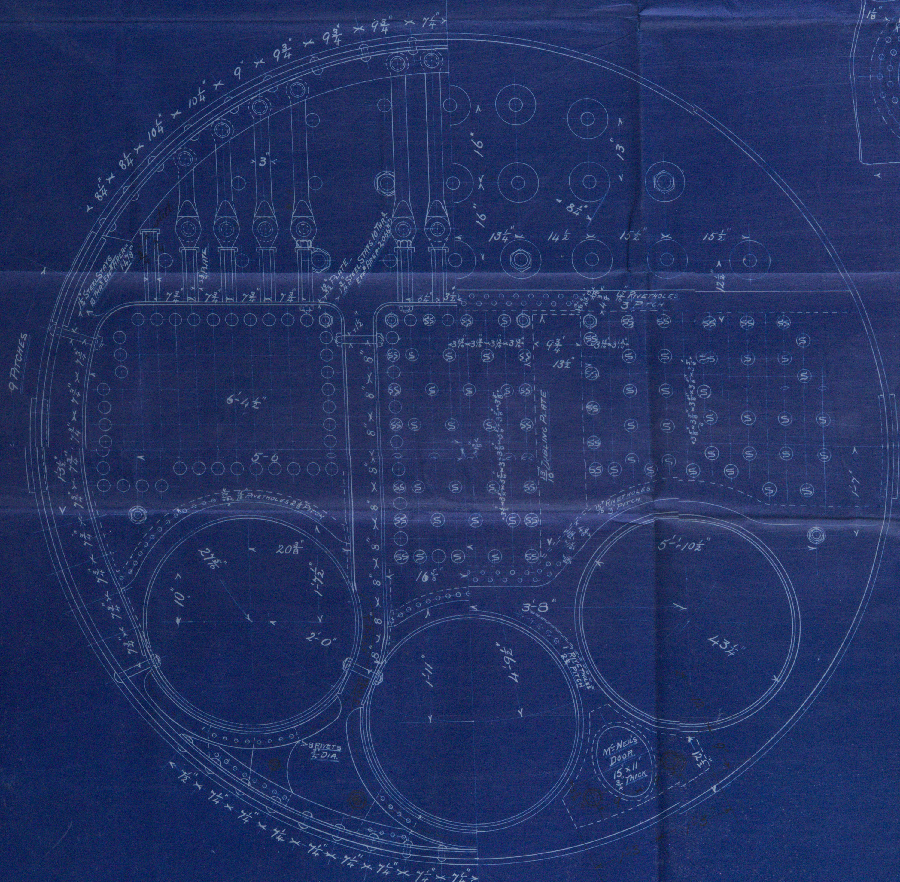
McNEIL'S DOOR & COMPENSATING RING DOOR 16 x 12 1/2" THICK
