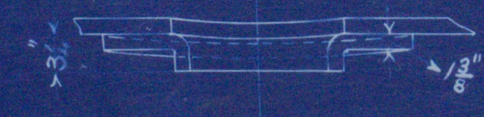
McNEIL'S DOOR & COMPENSATING RING DOOR 16 x 12 1/2" THICK
