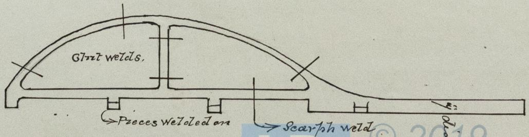
Rudder Frame Forging
