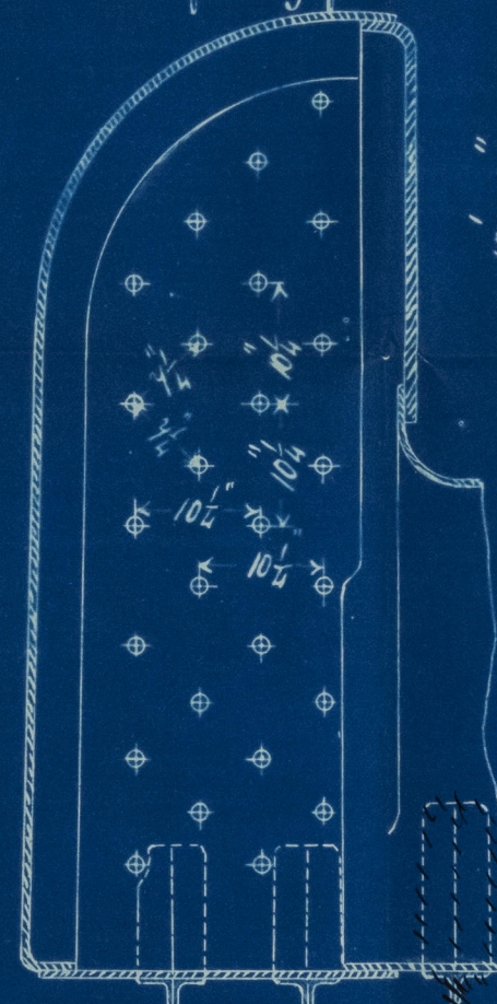
Arrangement of stays on outer sides of wing fire boxes
