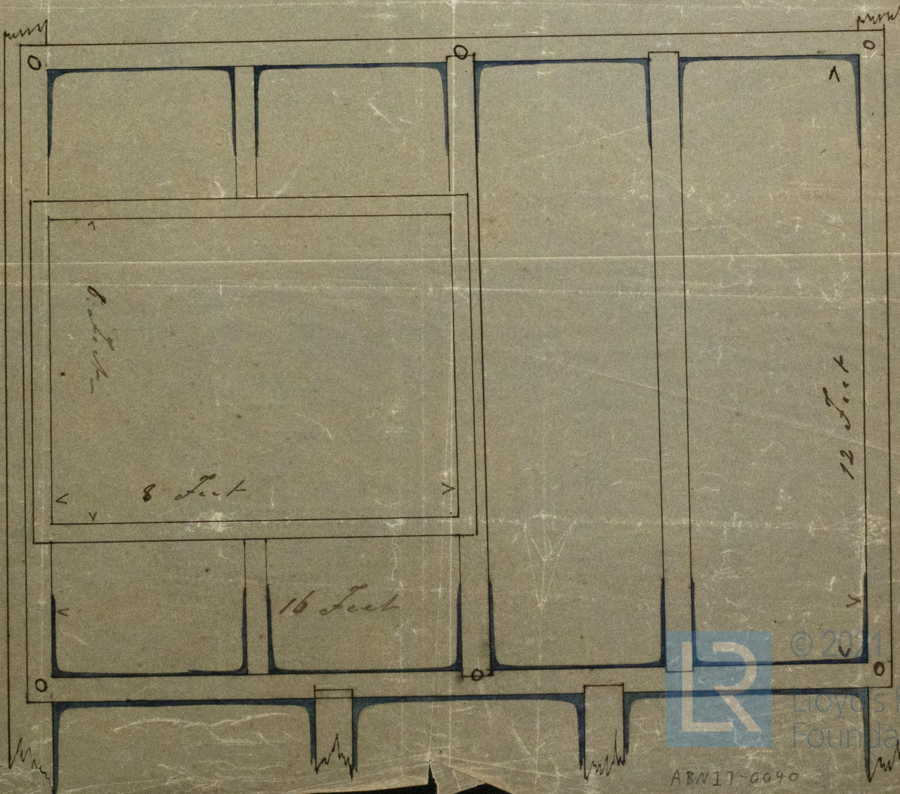
Main Hatchway of the Ship "Liba" of London.
