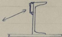
Side frames in tween deck fitted with  $3\frac{1}{2}$ " x  $3\frac{1}{2}$ " x .50" reverse bars, forming a 6" deep section, at frames 145 to 166, and at alternate frames from frame 140 to frame 9. Reverse bars efficiently connected at ends. ✓
