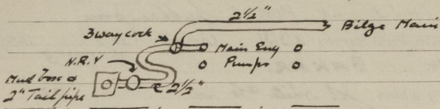
The connection to the fore hold (c) from the distribution box in the Engine Room is now led to a second distribution box in the Engine Room & thence to port & starboard of fore hold, both sections being through N.R.V.'s & 2" dia; This arrangement being required by the fitting of tanks in the hold.
