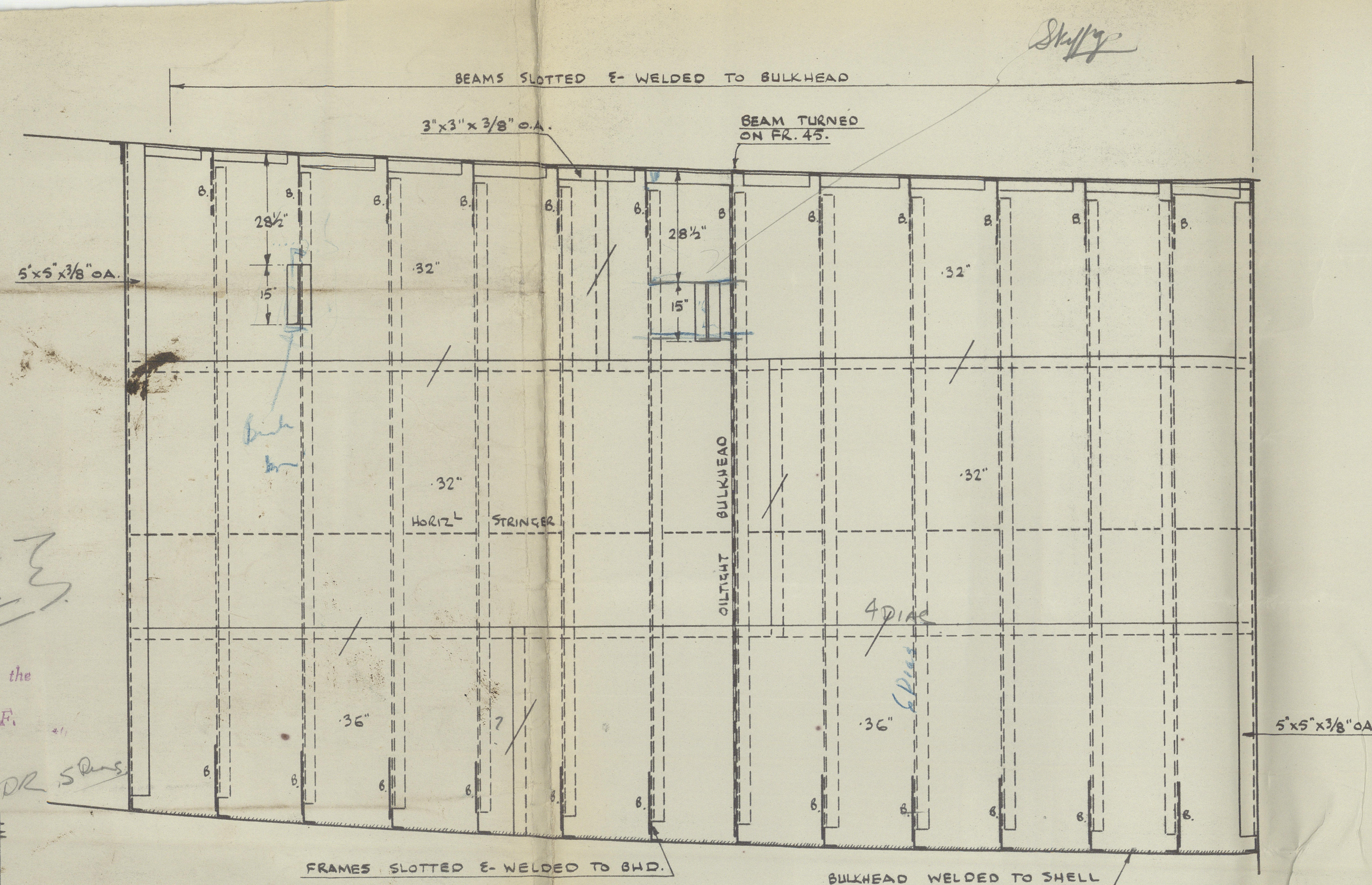
ELEVATION OF O.T. BULKHEAD 52. 3'-0" OFF & PORT & STARBOARD. DRAWN FOR PORT SIDE LOOKING TO PORT. STARBOARD SIDE SIMILAR. STIFFENERS - 6" x 3" x 3/8" O.A. (RIVETED).
