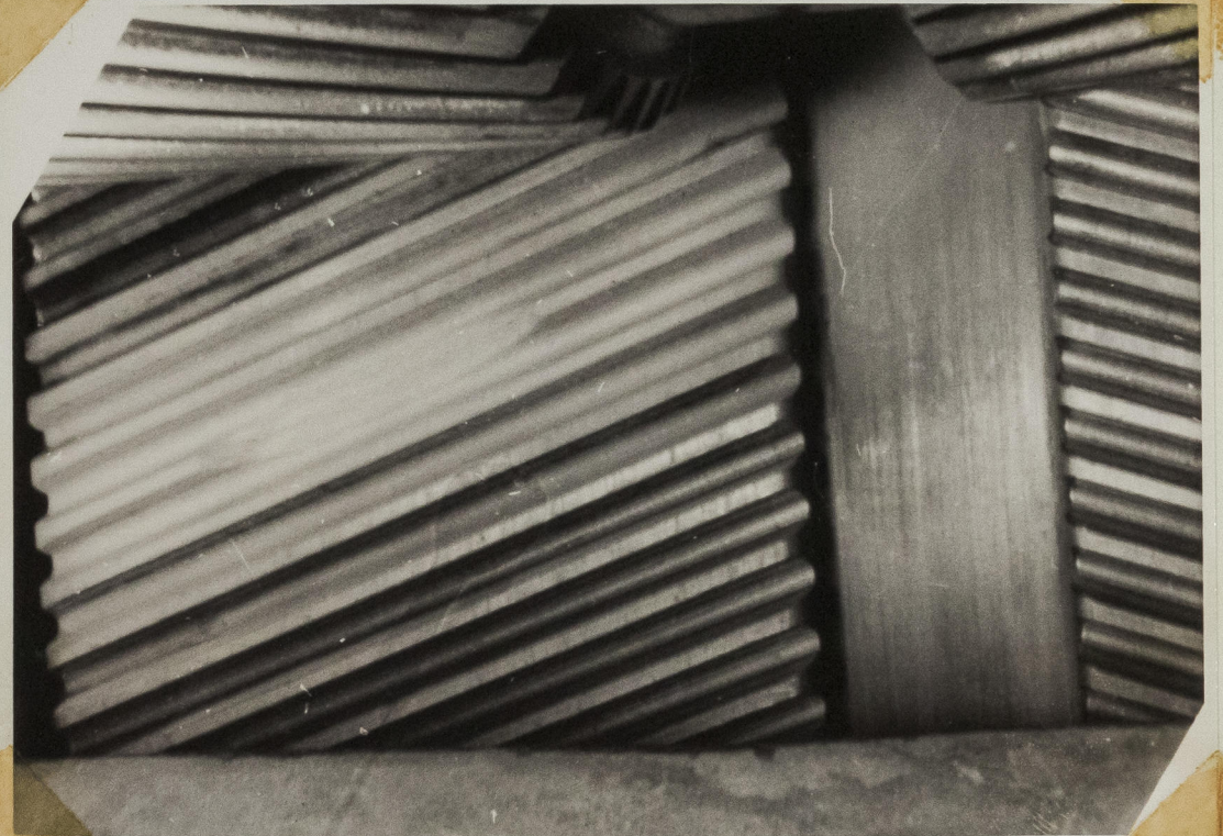
H.P. 1st Wheel aft Helix Dyecheck Inspection after Repaired.
