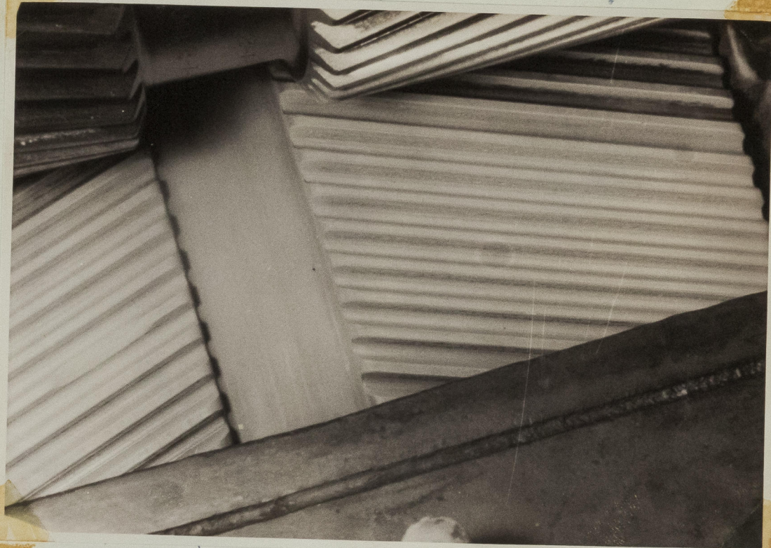
H.P. 1st Wheel Fore Helix Dyecheck Inspection after Repaired
