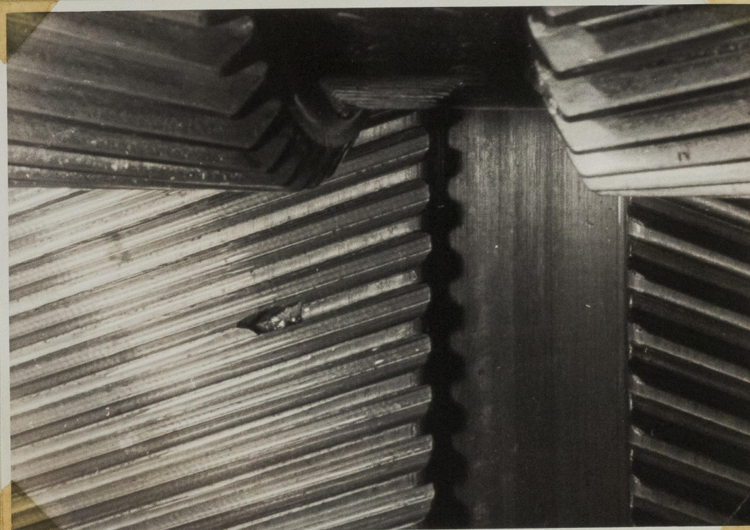
H.P. 1st Wheel aft Helix before Repair
