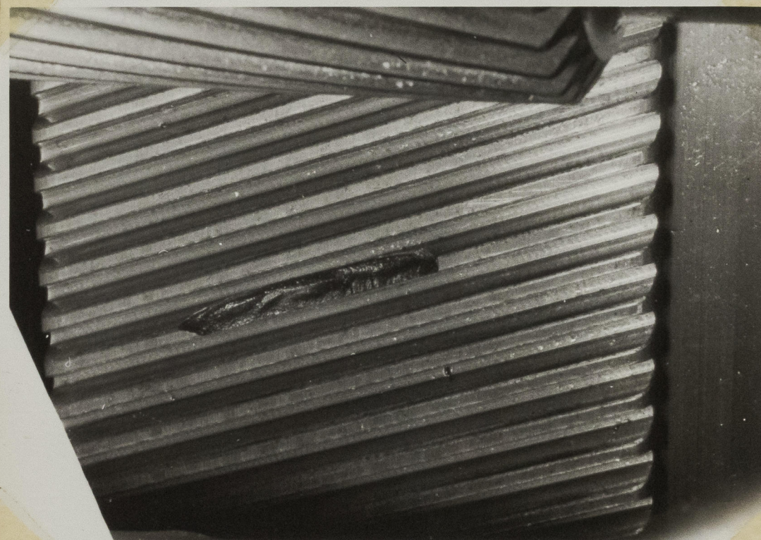
H.P. 1st Wheel aft Helix before Repair
