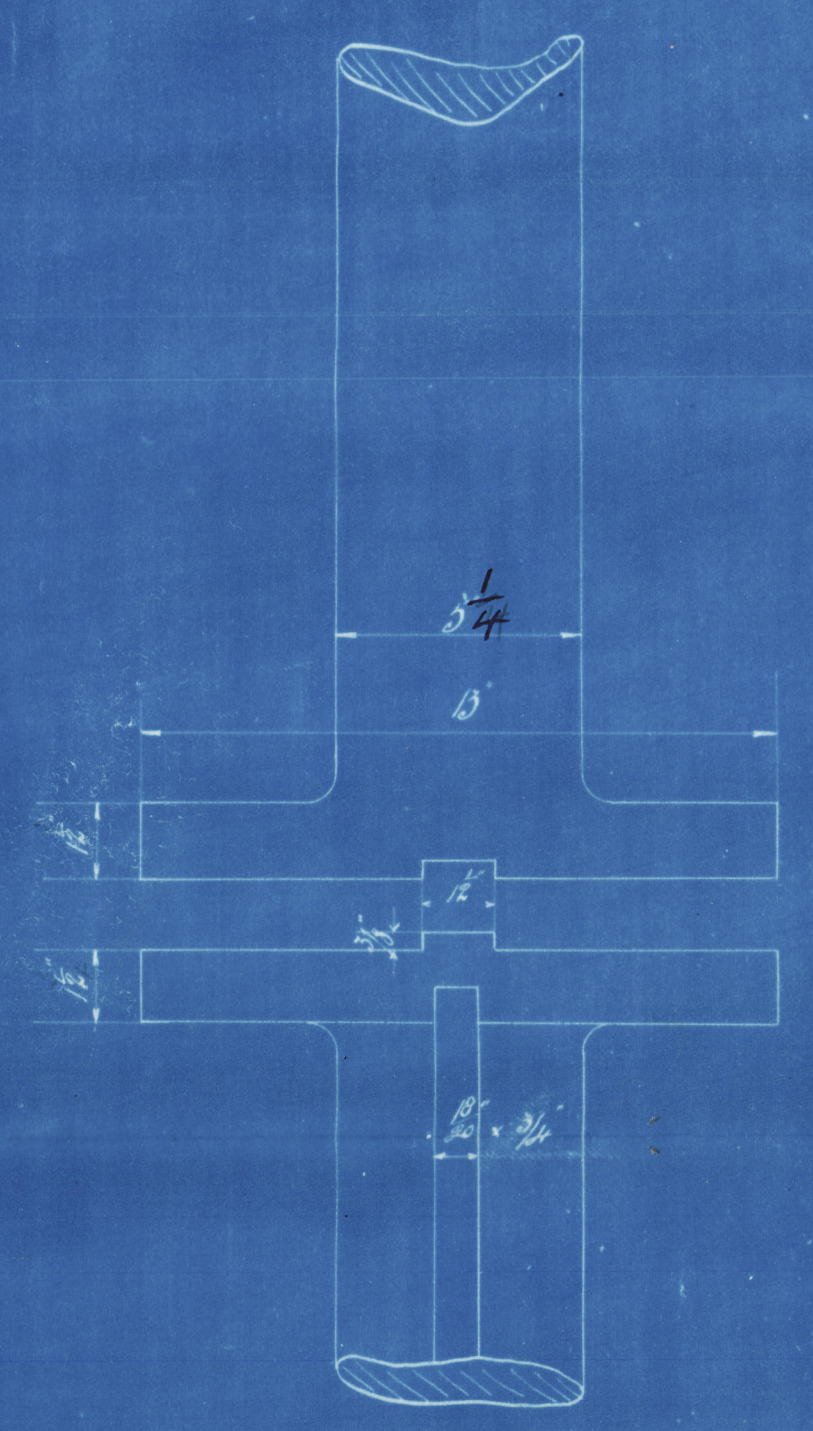
Detail of Coupling Scale 5' = One ft.
