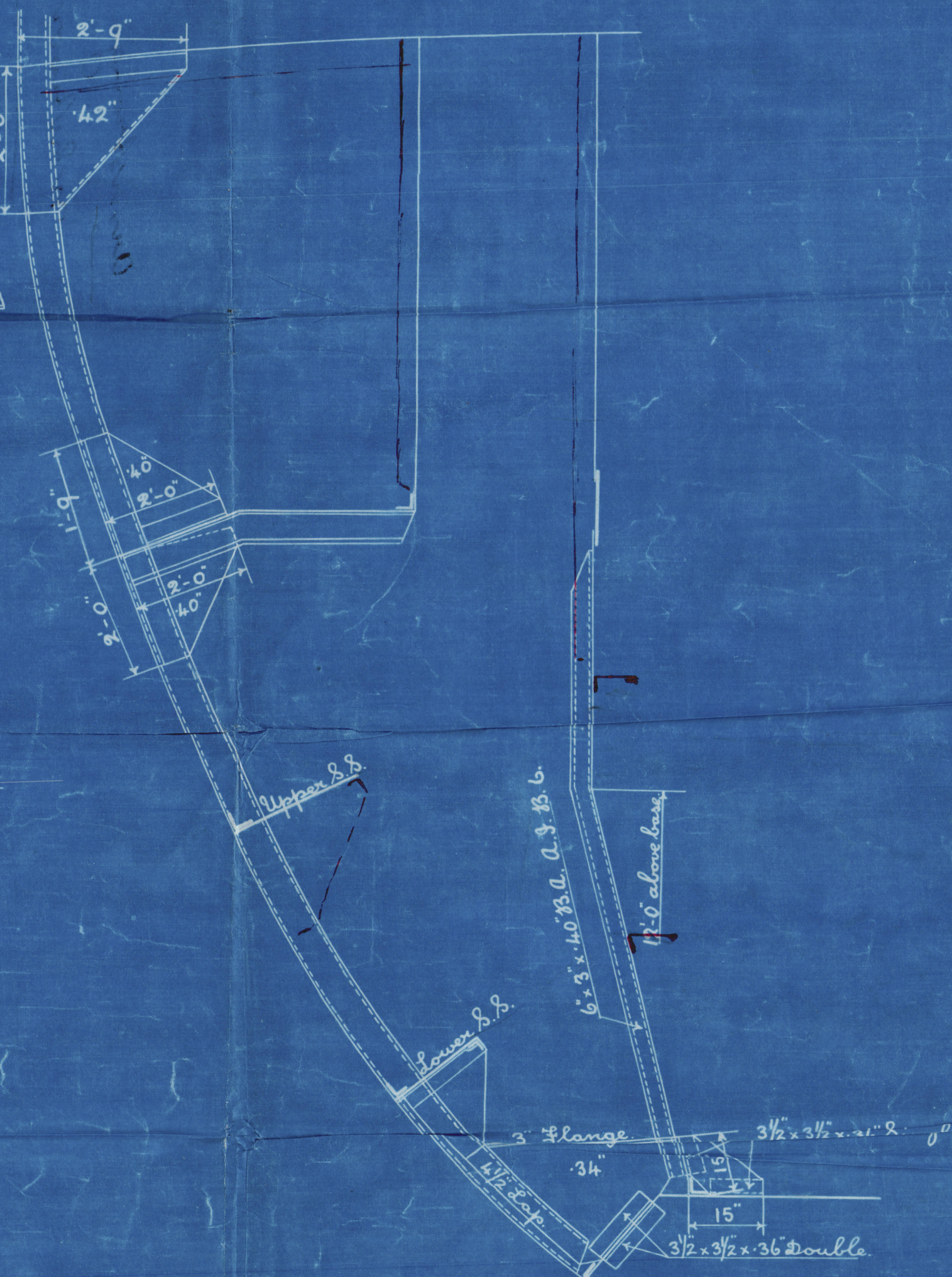
Detail of Upper Side Stringer in way of Ice Box
