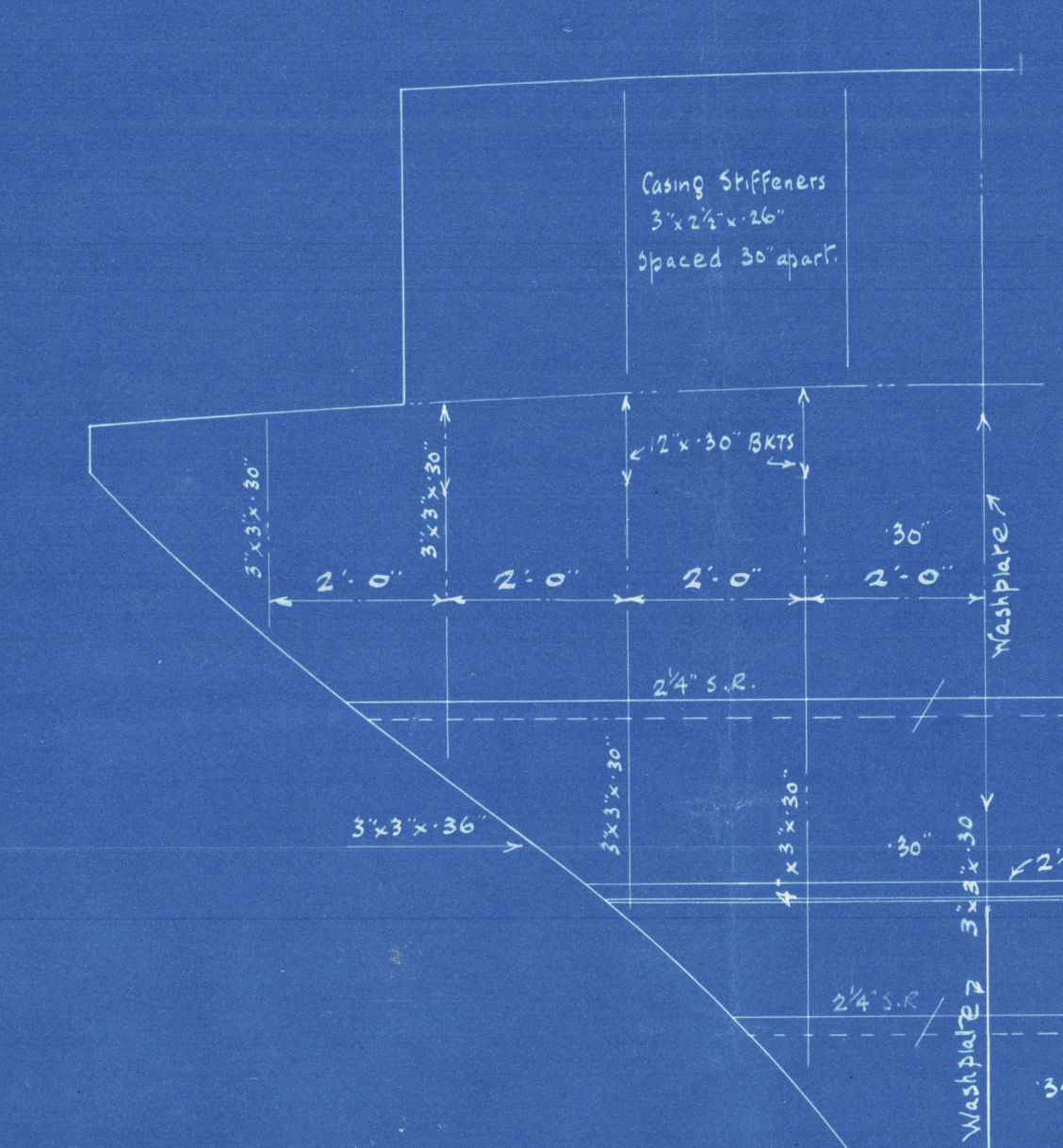
W.T. Bulkhead No 6 looking aft stiffeners on aft side
