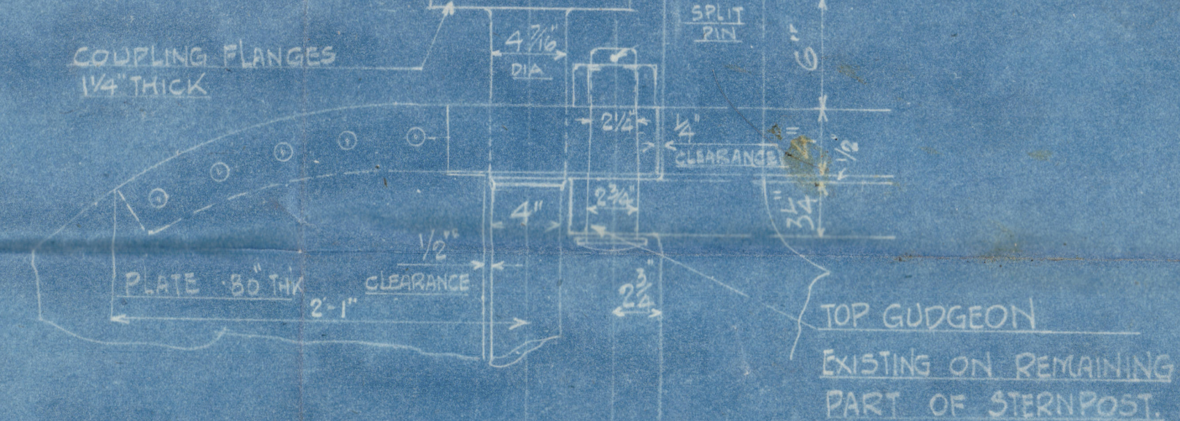
ELEVATION OF TOP PINTLE & GUDGEON ALSO COUPLING
