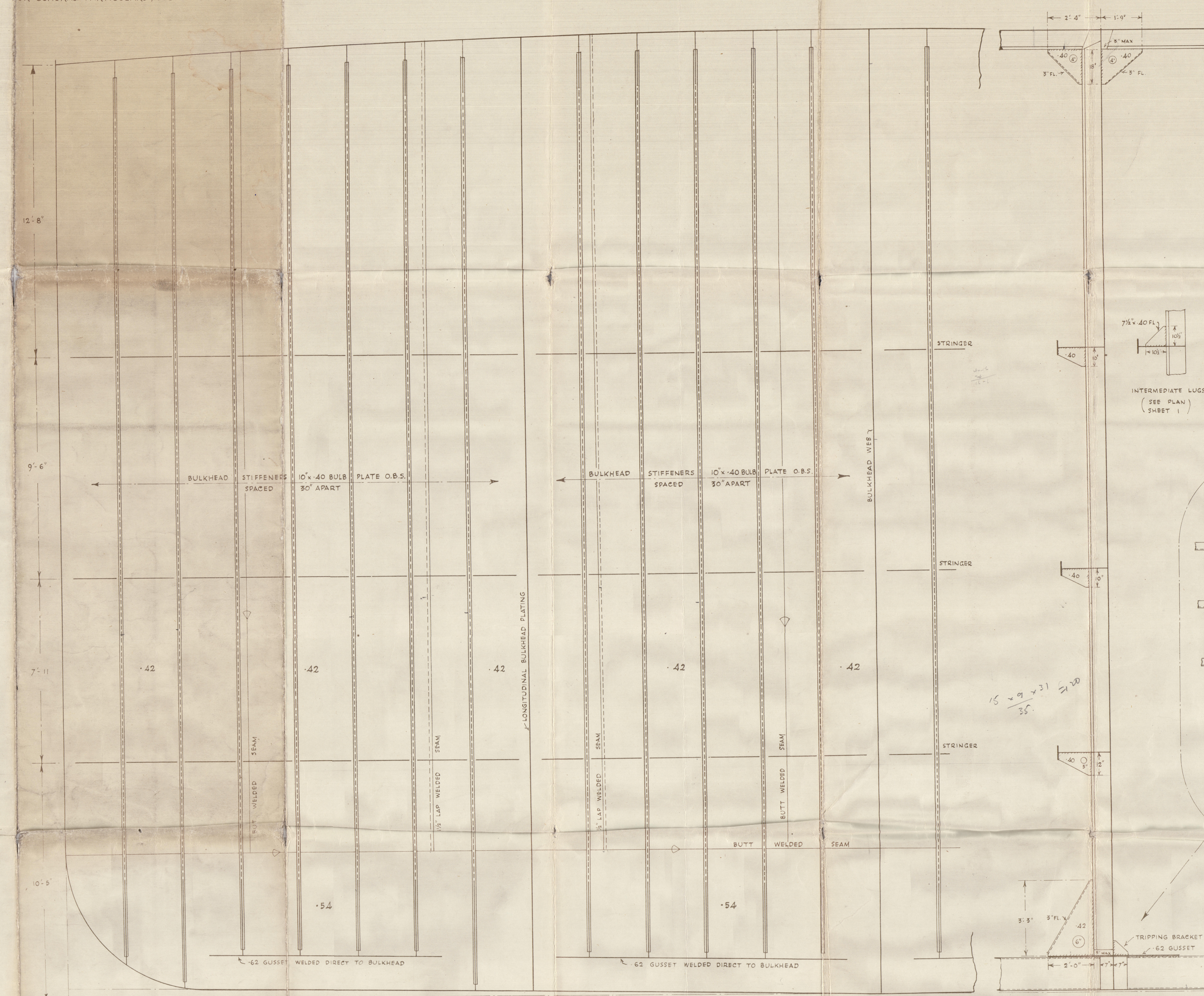
STIFFENERS IN CENTRE TANK & WHERE MARKED 'B' IN WING TANKS
