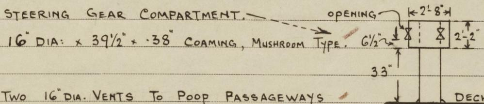
POOP DECK. TWO 16" DIA. VENTS TO POOP PASSAGEWAYS AT AFTER END P&S, COAMINGS INCREASED IN HEIGHT TO 8'-9" x .38", STAYED TO BOAT DECK. CLOSED WITH WOOD PLUGS AND CANVAS COVERS. ✓
