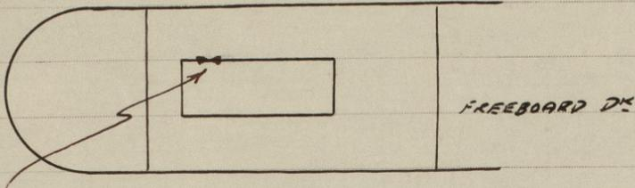
New steel door in machinery casing (port side) with lock, 2 hinges
