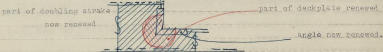
From F.P. bulkhead (peak overpressed; airpipe found plugged) 3rd strake from bottom renewed; 4th and 5th strake released, faired and riveted; lugs from both stringers on bulkhead renewed.
