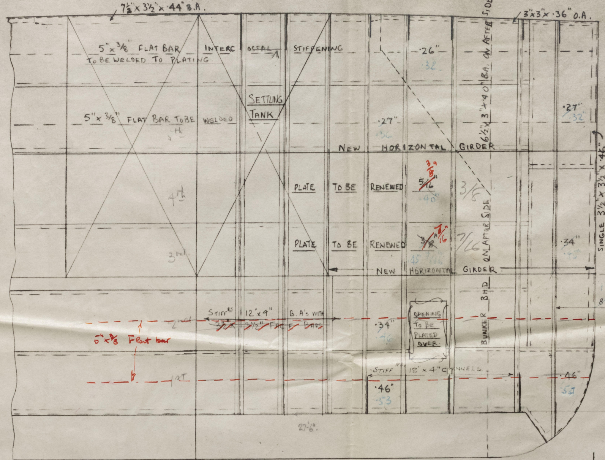
PLAN OF UPPER HORIZONTAL GIRDER
