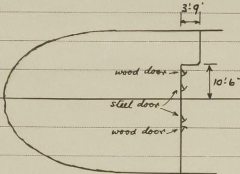
Poop front steel bulkhead extended on port side as shown in sketch and 2 steel doorways blanked off.
