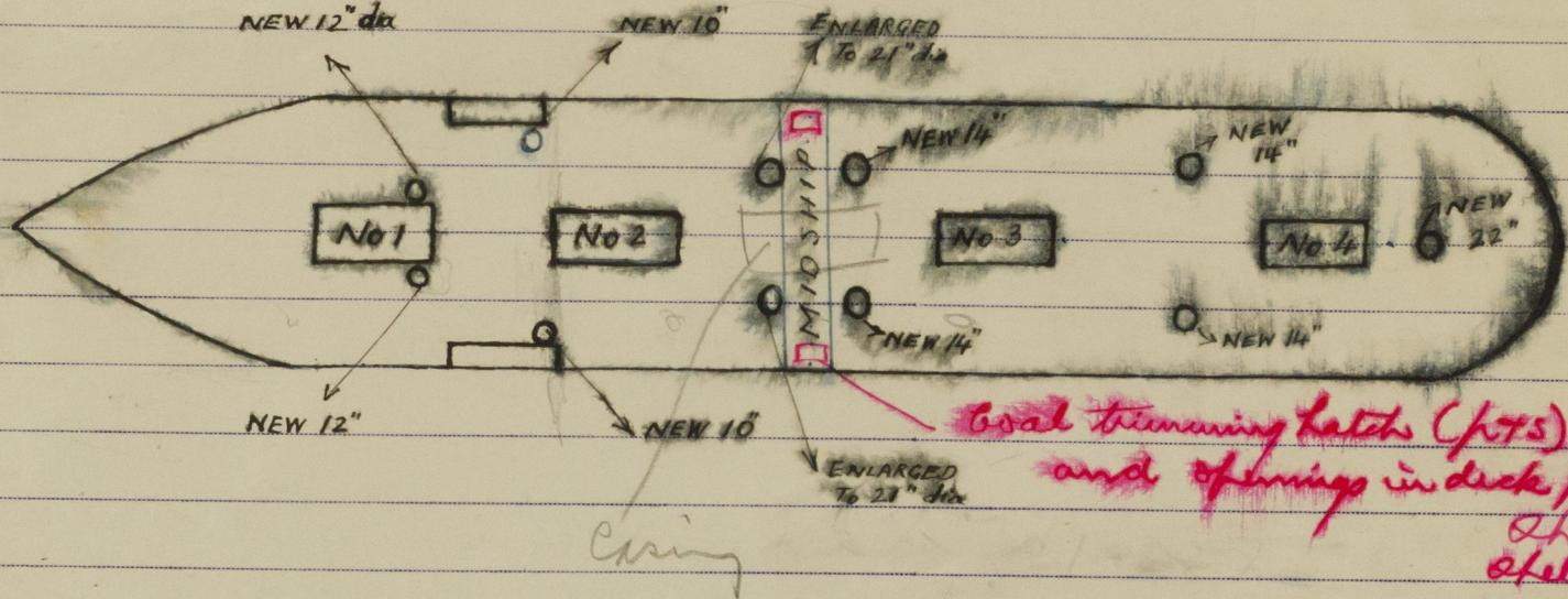
All these ventilator coamings are to Rule requirements and the plugs and covers are new and in good order. All these ventilators are on the shelter deck and are for additional ventilation to the shelter deck space above the freeboard deck. The coal trimming hatches on the shelter deck, midships, have been removed, one port one starboard, and the openings in the deck plated over and sheathed.
