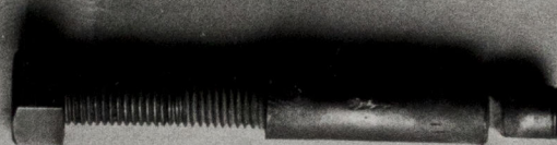
DISCHARGE VALVE GUIDE FWD. FEED PUMP
