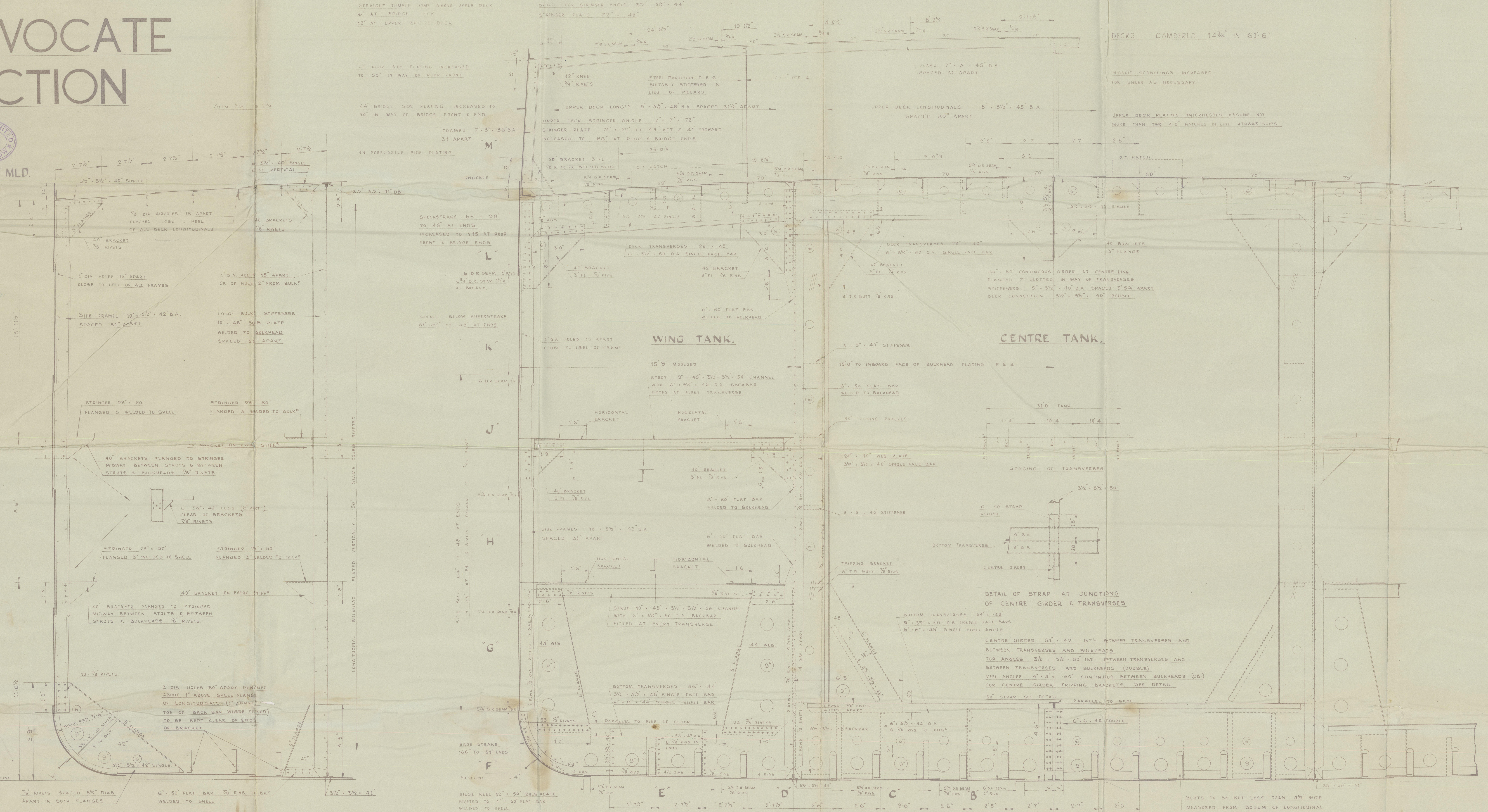
SECTION THRO' WING TANKS AT INTERMEDIATE FRAMES LOOKING AFT.
