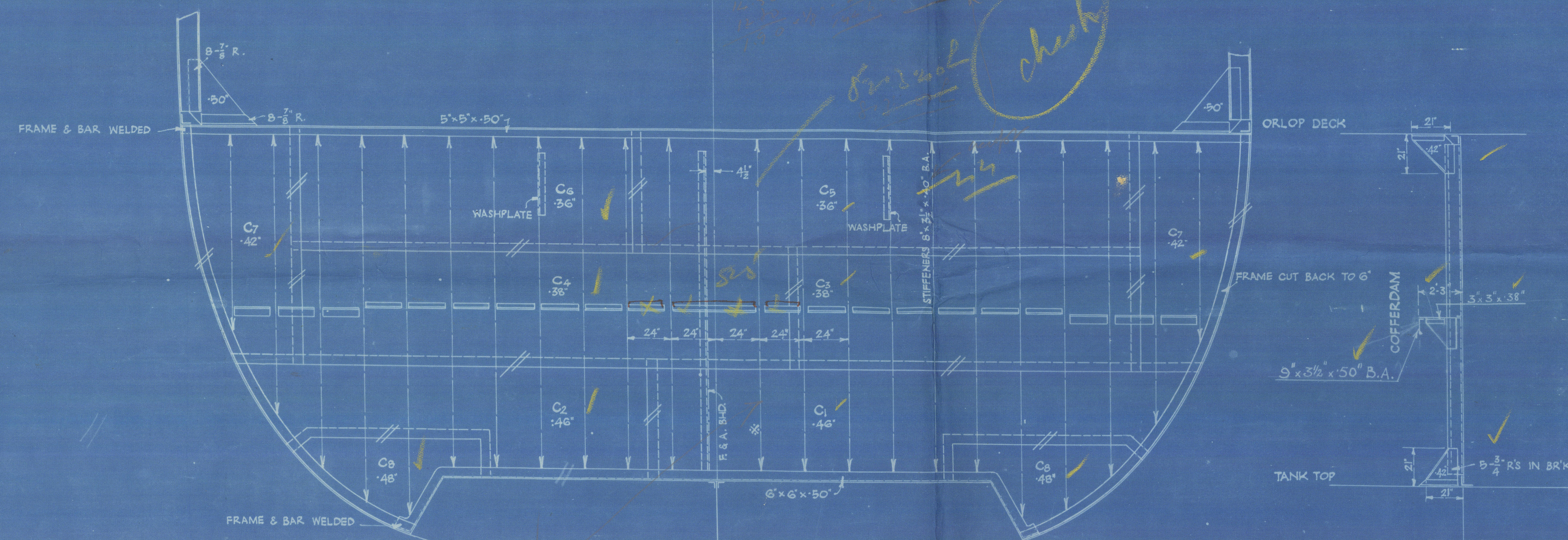
BULKHEAD ON FRAME 181 LOOKING FORW.
