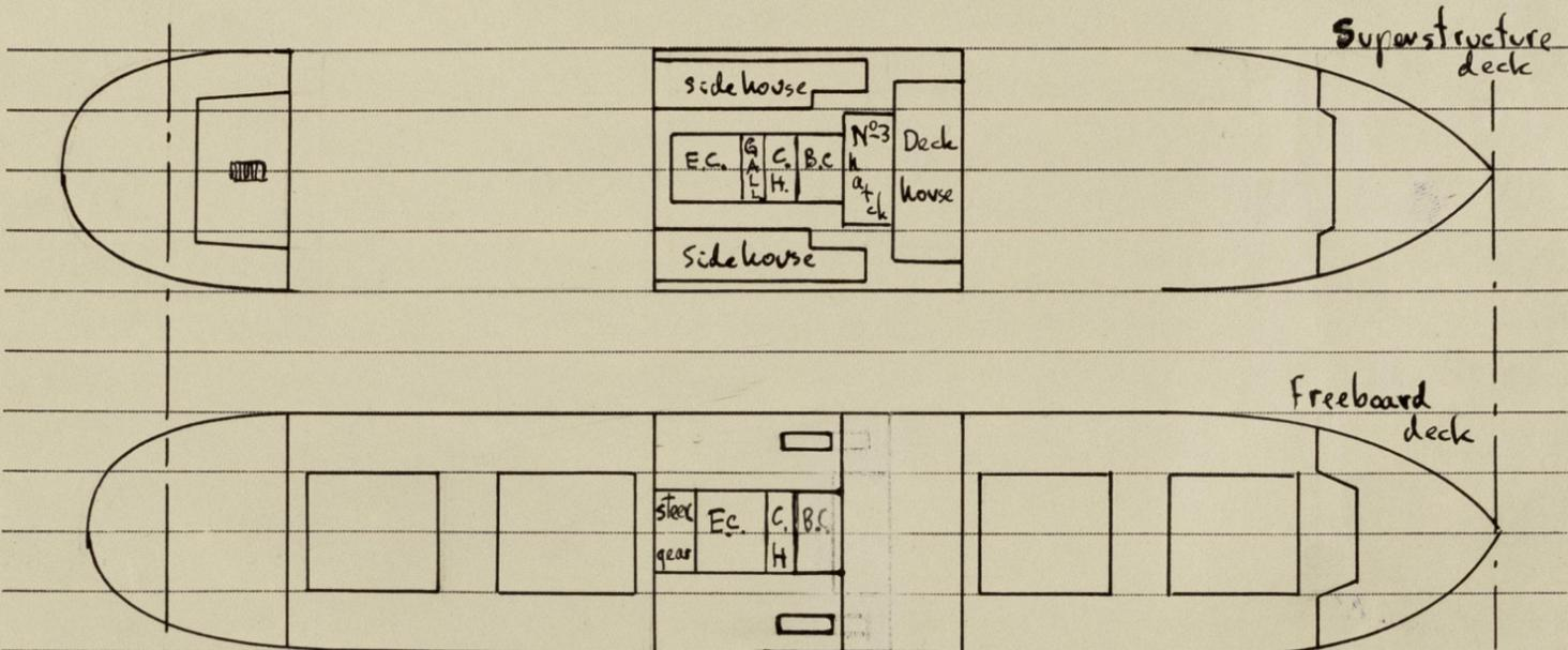
Companionway and skylight on poopdeck cut away and companion enclosed in efficiently constructed steel deck house.
