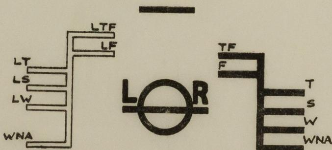
I hereby certify that this ship has been surveyed and the freeboards and load lines shown above have been assigned in accordance with the Convention.
