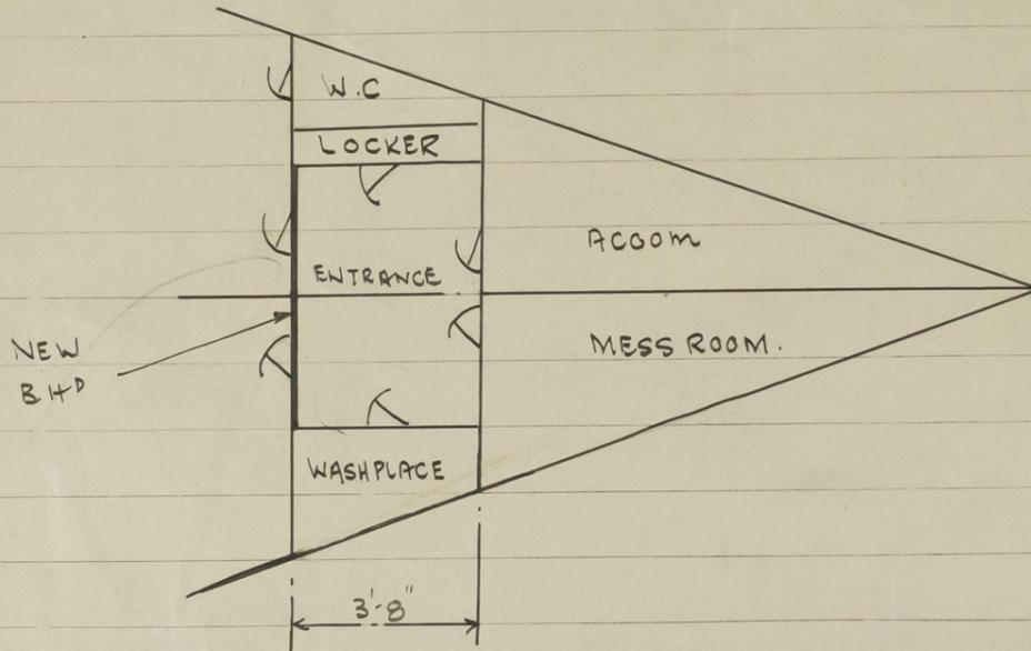
Poop front bulkhead fitted with hinged wood door at middleline of ship 4'7" x 28" x 18" sill, with spring lock manipulated from both sides.
