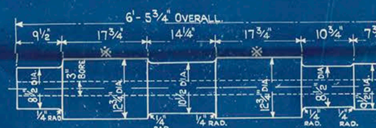
L.P. PINION SHAFT.
