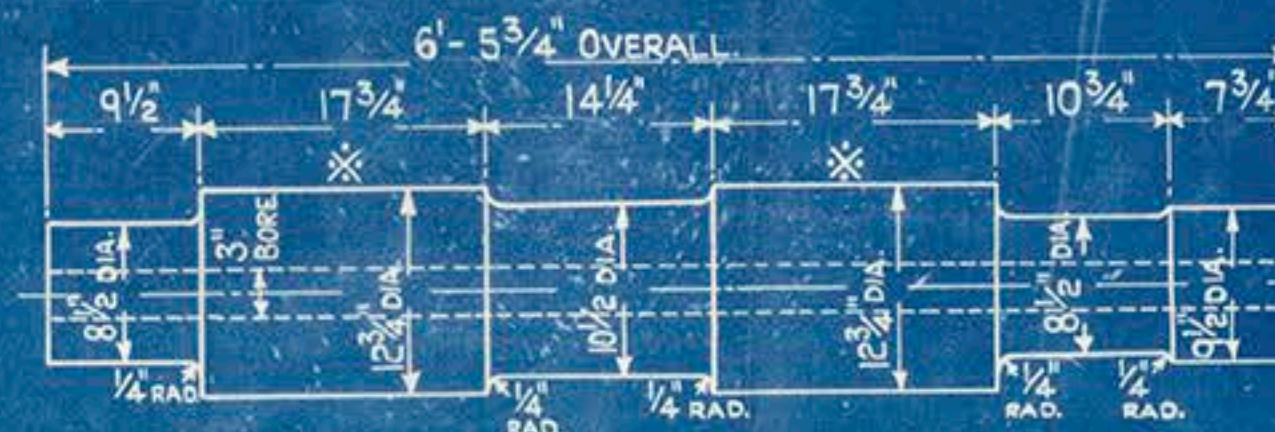
L.P. PINION SHAFT. SCALE: 1" TO 1 FOOT.
